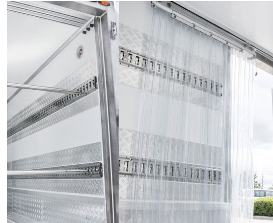
Internal wall tracks
