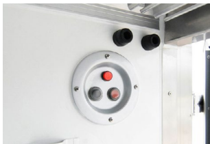
Light Switch and Internal Alarm
